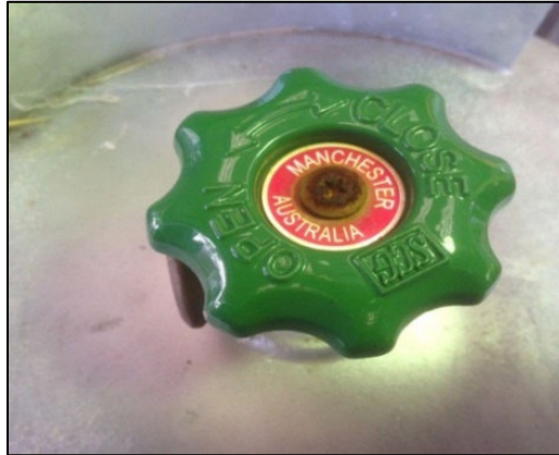
Figure 26. Exchangeable gas cylinder showing green tap with 'OPEN' and 'CLOSE' markings
