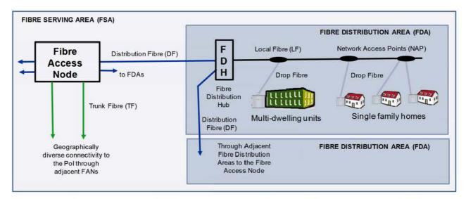
The Stage 1 plan is to provide a detailed design for a number of Fibre Serving Area Modules (FSAM), where each module will be limited to a maximum of 16 Fibre Distribution Areas (FDAs) which will result in approximately 3,200 premises. The model FSAM shown below will be utilised as the basis for the design, with an inner and outer distribution fibre loop provided to allow the integration of point to point services and minimise the impact of fibre breaks.
