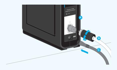
Connect the other end of the white cable B to the back of your **nbn**<sup>™</sup> connection box A Connect the power adaptor c to the back of the **nbn**<sup>™</sup> connection box A
